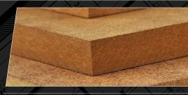
Medium-density fibreboard (MDF) is an engineered wood product made by breaking down hardwood or softwood residuals into wood fibres, often in a defibrator, combining it with wax and a resin binder, and forming it into panels by applying high temperature and pressure. MDF is generally more dense than plywood.
